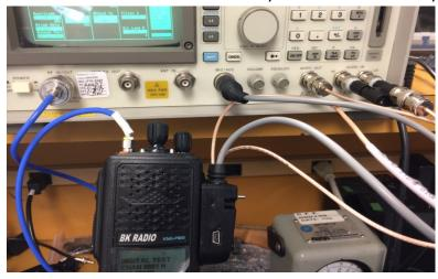
i. On HP8920, in RX Test mode, place the cursor to AF ANL under To Screen box then press the cursor control knob. It should go to the next screen.
