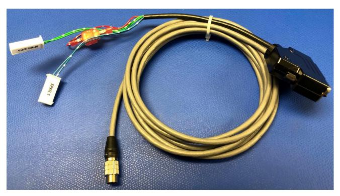
2. Plug in the DB25 connector to the accessory port of the KNG Mobile radio then plug in the KAA0276 Speaker Mic to the Hirose connector in the other end of the extension cable.
