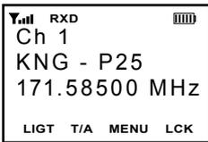
When a signal is received, the unprogrammable top line of the display indicates the current channel's operating mode. RXA = analog, RXD = digital.
