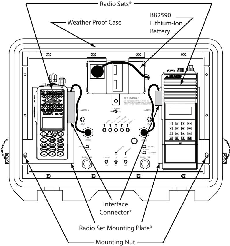
\*Interface connectors and mounting plates are dependant radio set type.
